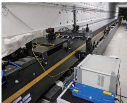
图 12 光频扫描干涉测距精度测试现场图 Fig.12 Accuracy testing of absolute distance measurement based on frequency scanning interferometry
