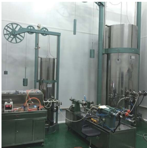
图6 对小流量高压仪表的检定/校准 Fig.6 Verification / calibration of small-flow high-pressure instruments
